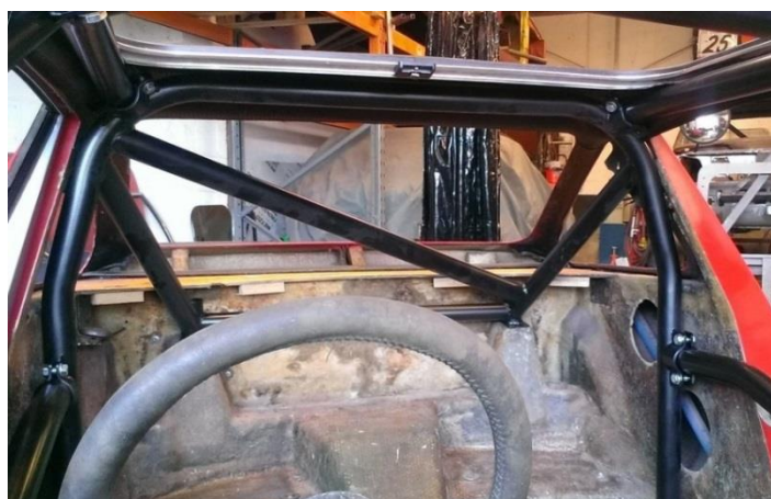
A steel cage being fitted to a Clan by Malkin Motorsport
