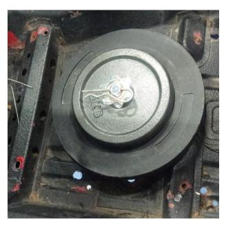
Regulations covering the installation of ballast can be found in (J)5.15.2, which states that the ballast must be attached to the shell/chassis via at least four mounting points using bolts of a minimum 8mm diameter, there is also a requirement for 400mm<sup>2</sup> counter-plates of 3mm thick steel for each mounting point.
