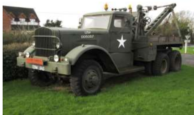
1941 'Ward LaFrance M1' Heavy Wrecker Truck 45mph Continental 8.2 litre 6-cylinder petrol engine 145bhp US Army and British REME in the Middle East & Italy
