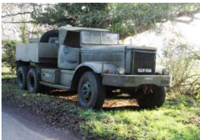
1943 M20 'Diamond T 980' Tank Transporter 23mph Hercules 14.7 litre 6-cylinder diesel engine 185bhp Used by the British Army mainly in N.Africa
